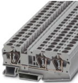
Feed-through terminal block, Connection method: Spring-cage connection, Cross section: 0.2 mm 2 - 10 mm 2 , AWG: 24 - 8, Width: 8.2 mm, Color: gray, Mounting type: NS 35/7,5, NS 35/15
