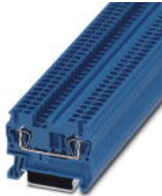
Feed-through terminal block, Connection method: Spring-cage connection, Cross section: 0.08 mm 2 - 4 mm 2 , AWG: 28 - 12, Width: 5.2 mm, Color: blue, Mounting type: NS 35/7,5, NS 35/15
