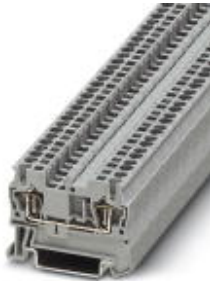
Feed-through terminal block, Connection method: Spring-cage connection, Cross section: 0.08 mm 2 - 4 mm 2 , AWG: 28 - 12, Width: 5.2 mm, Color: gray, Mounting type: NS 35/7,5, NS 35/15
