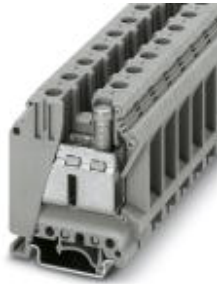
Feed-through terminal block, Connection method: Screw connection, Cross section: 0.75 mm 2 - 50 mm 2 , AWG: 18 - 1/0, Width: 15.1 mm, Color: gray, Mounting type: NS 35/7,5, NS 35/15, NS 32
