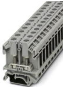
Bolt connection terminal block, Connection method: Bolt connection, Cross section: 0.1 mm 2 - 6 mm 2 , AWG: 26 - 10, Width: 11 mm, Color: gray, Mounting type: NS 35/7,5, NS 35/15, NS 32
