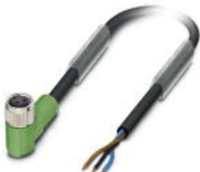
Sensor/Actuator cable, 3-position, PUR halogen-free, black-gray RAL 7021, free cable end, on Socket angled M8, Cable length: 10 m
