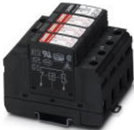
Surge voltage arrester combination 4-channel (in the 3+1 circuit), for mounting on NS 35/7.5, voltage 230 V AC
