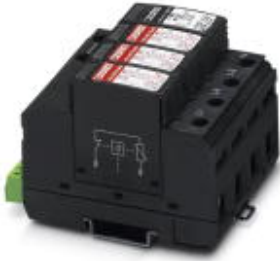
Surge voltage arrester consisting of base element with remote indicator contact and ground connectors, for mounting on NS 35/7.5, nominal voltage: 230 V AC, 3 + 1 circuit
