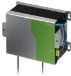
Power storage device, lead AGM, VRLA technology, 24 V DC, 12 Ah. Connection via pin cable lug, 14 mm.
