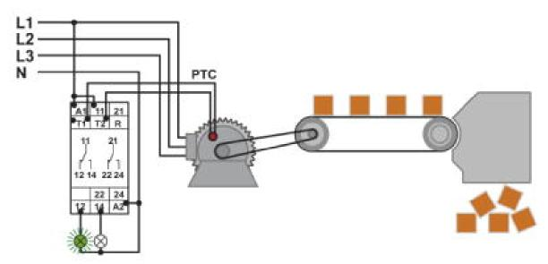
Monitoring of motor winding temperatures
