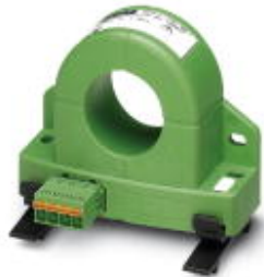
Universal current transducer, for measuring AC, DC, and distorted currents, 0 ... 100 A input current, 4 ... 20 mA output
