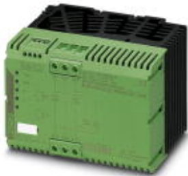
Three-phase solid-state reversing contactor with 24 V DC input, 16 A output current, zero voltage switch, optionally with thermal fuse
