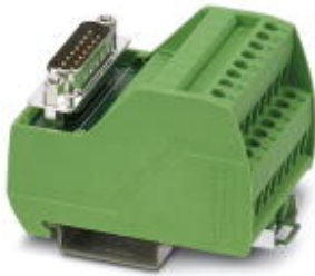
VARIOFACE module, with screw connection and male D-Subminiature pin strip, for mounting on NS 35 rails, 15-pos.
