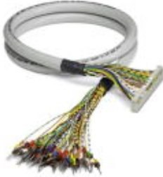
Round cable assembled with a 20-pos. socket strip and an open end. On the open end, the wires are labeled with 1 to 20 and have ferrules, cable length: 3 m
