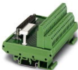
VARIOFACE module, with screw connection and D-Subminiature socket strip, for mounting on NS 35/7.5 or NS 32, 9-pos.
