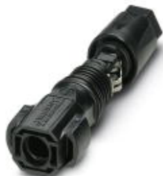
Photovoltaic connector, Nominal current: 40 A, Nom. voltage: 1100 V, Connection type: Spring-cage, Color: black, Can only be released using a tool
