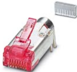
RJ45 male insert, CAT6, 8-pos., shielded, IDC displacement connection, for litz wire AWG 25 ... 24 and solid wires AWG 24, with strain relief
