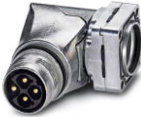
Device connector, front mounting, angled rotatable, SPEEDCON locking, M17, Number of positions: 3+PE, Type of contact: Male connector, Crimp connection, Axial O-ring, 4xØ2,7, shielded: Yes, Flange dimensions: 21.6 mm x 21.6 mm
