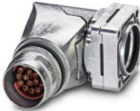
Device connector, front mounting, angled rotatable, SPEEDCON locking, M17, Number of positions: 17, Type of contact: Socket, Crimp connection, Axial O-ring, 4xØ2,7, shielded: Yes, Flange dimensions: 21.6 mm x 21.6 mm
