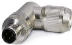
Bus system connector, Ethernet CAT5, Ethernet CAT5e, 4-position, shielded, Plug angled M12, D-coded, Insulation displacement connection, Knurl material: Nickel-plated brass, External cable diameter 4 mm ... 8 mm
