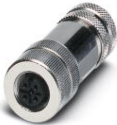
Bus system connector, female straight, 5-pos., M12, shielded, gold-plated contacts, A-coded, screw connection, metal knurl, cable screw connection Pg9
