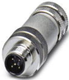
Bus system connector, male, straight, 5-pos., M12, shielded, gold-plated contacts, A-coded, screw connection, metal knurl, cable screw connection Pg9
