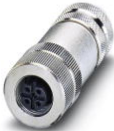
Bus system connector, female, straight, 5-pos., M12, shielded, gold-plated contacts, B-coded, screw connection, metal knurl, cable screw connection Pg9
