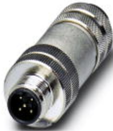
Bus system plug-in plug, male straight, 5-pos., M12, shielded, gold-plated contacts, B-coded, screw connection, metal knurl, cable screw connection Pg9
