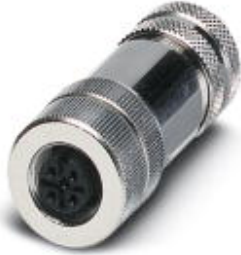
Sensor/actuator connector, female, straight, 4-pos., M12, shielded, A-coded, screw connection, metal knurl, cable screw connection Pg7
