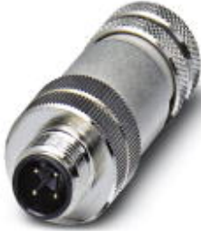
Sensor/actuator connector, male, straight, 4-pos., M12, shielded, A-coded, screw connection, metal knurl, cable screw connection Pg7
