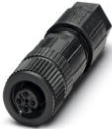
Connector, 4-position, Socket straight M12, A-coded, Spring-cage connection, Knurl material: Plastic, External cable diameter 4 mm ... 8 mm
