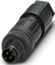
Connector, 4-position, Plug straight M12, A-coded, Spring-cage connection, Knurl material: Plastic, External cable diameter 4 mm ... 8 mm
