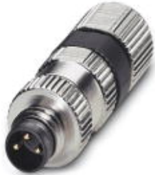
Sensor/actuator connector, male, straight, 3-pos., M8, Piercecon ® , metal knurl, cable diameter max. 5 mm
