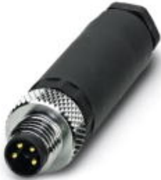
Connector, 4-position, Plug straight M8, A-coded, Screw connection, Knurl material: Nickel-plated brass, External cable diameter 3.5 mm ... 5 mm
