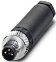
Connector, 3-position, Plug straight M8, A-coded, Screw connection, Knurl material: Nickel-plated brass, External cable diameter 3.5 mm ... 5 mm
