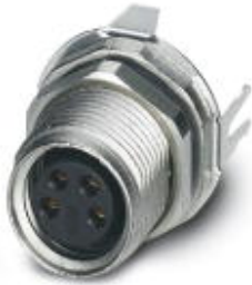
Sensor/actuator flush-type connector, socket, 4-pos. M8, rear/screw mounting with M10 fastening thread, with straight solder connection
