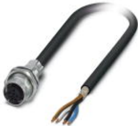
Flush-type socket, shielded, 4-pos., M12, A-coded, rear/screw mounting with M16 thread, with 1 m cable, 4 x 0.34 mm 2
