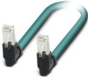
Patch cable, CAT5e, 4-pair, shielded, line, assembled at both ends with angled RJ45/IP20 heads, length: 0.3 m
