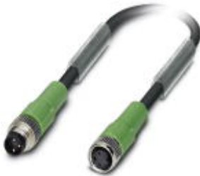
Sensor/Actuator cable, 3-position, PUR halogen-free, black-gray RAL 7021, Plug straight M8, on Socket straight M8, Cable length: 1 m
