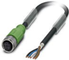
Sensor/Actuator cable, 5-position, PUR halogen-free, black-gray RAL 7021, shielded, free cable end, on Socket straight M12, A-coded, Cable length: 5 m
