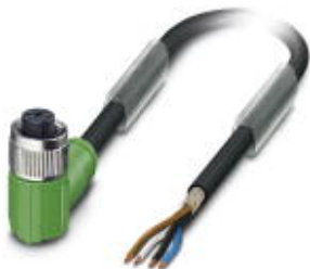
Sensor/Actuator cable, 4-position, PUR halogen-free, black-gray RAL 7021, shielded, free cable end, on Socket angled M12, A-coded, Cable length: 5 m
