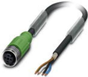
Sensor/Actuator cable, 4-position, PUR halogen-free, black-gray RAL 7021, shielded, free cable end, on Socket straight M12, A-coded, Cable length: 5 m
