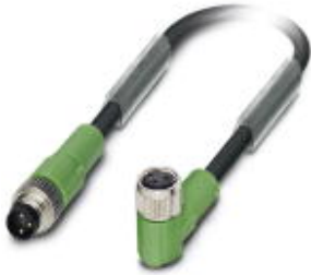
Sensor/Actuator cable, 3-position, PUR halogen-free, black-gray RAL 7021, Plug straight M8, on Socket angled M8, Cable length: 0.6 m
