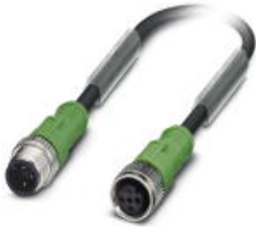
Sensor/Actuator cable, 3-position, PUR halogen-free, black-gray RAL 7021, Plug straight M12, A-coded, on Socket straight M12, A-coded, Cable length: 3 m
