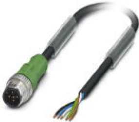
Sensor/Actuator cable, 5-position, PUR halogen-free, black-gray RAL 7021, Plug straight M12, A-coded, on free cable end, Cable length: 5 m
