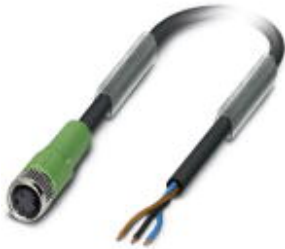
Sensor/Actuator cable, 3-position, PUR halogen-free, black-gray RAL 7021, free cable end, on Socket straight M8, Cable length: 1.5 m
