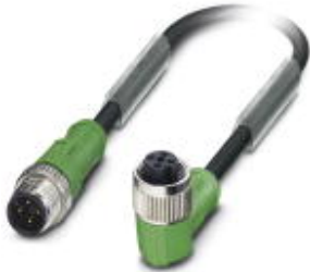
Sensor/Actuator cable, 4-position, PUR halogen-free, black-gray RAL 7021, Plug straight M12, A-coded, on Socket angled M12, A-coded, Cable length: 3 m
