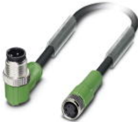
Sensor/Actuator cable, 3-position, PUR halogen-free, black-gray RAL 7021, Plug angled M12, A-coded, on Socket straight M8, Cable length: 10 m
