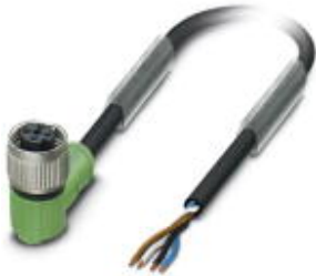
Sensor/Actuator cable, 4-position, PUR halogen-free, black-gray RAL 7021, free cable end, on Socket angled M12 SPEEDCON, A-coded, Cable length: 5 m
