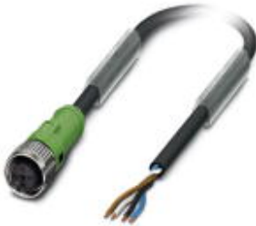
Sensor/Actuator cable, 4-position, PUR halogen-free, black-gray RAL 7021, free cable end, on Socket straight M12 SPEEDCON, A-coded, Cable length: 5 m
