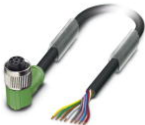
Sensor/Actuator cable, 8-position, PUR halogen-free, black-gray RAL 7021, free cable end, on Socket angled M12, A-coded, Cable length: 10 m
