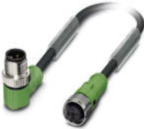
Sensor/Actuator cable, 4-position, PUR halogen-free, black-gray RAL 7021, Plug angled M12 SPEEDCON, A-coded, on Socket straight M12 SPEEDCON, A-coded, Cable length: 1.5 m
