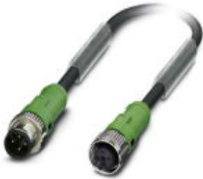
Sensor/Actuator cable, 4-position, PUR halogen-free, black-gray RAL 7021, Plug straight M12 SPEEDCON, A-coded, on Socket straight M12 SPEEDCON, A-coded, Cable length: 3 m
