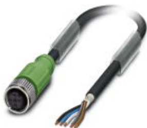
Sensor/Actuator cable, 5-position, PUR halogen-free, black-gray RAL 7021, shielded, free cable end, on Socket straight M12, A-coded, Cable length: 10 m
